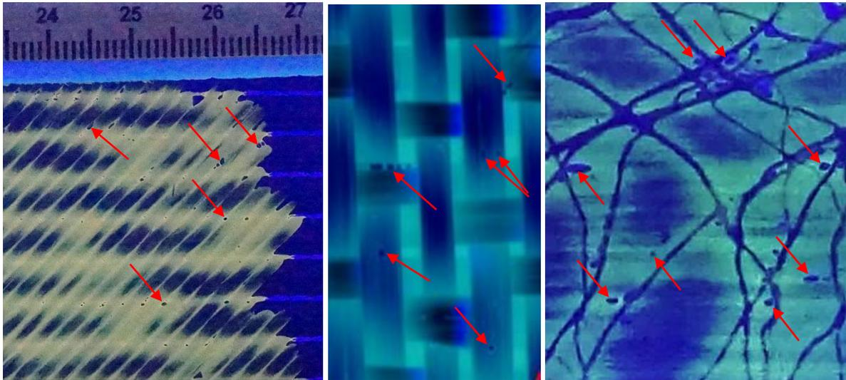
**Figure 1:** Example void images with carbon reinforcements: (from left to right) biax non-crimped fabric, satin weave, spread-tow weave with binder beads on surface. Arrows mark example void locations.
