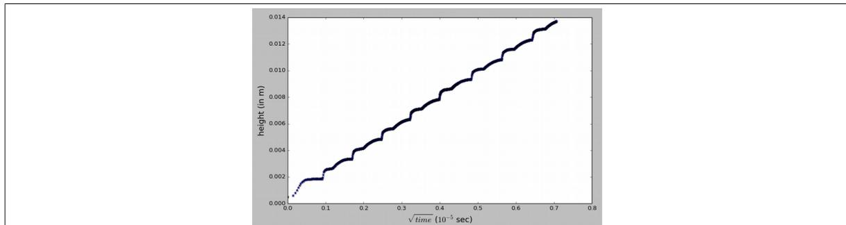
**Figure 2:** Height of the resin interface as a function of square root of time (9 fibres in the domain).
