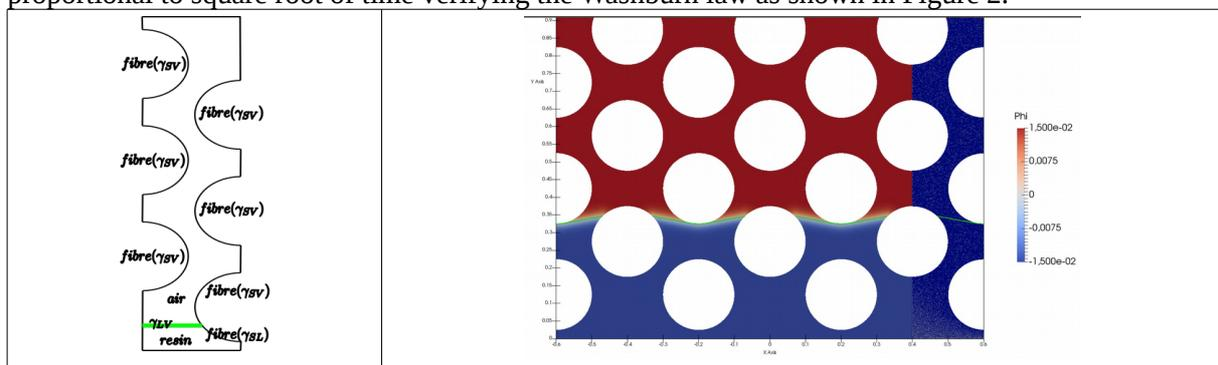
**Figure 1:** Boundary conditions and a snapshot during the simulation (axis x and y in cm) – 6 fibres in the domain
