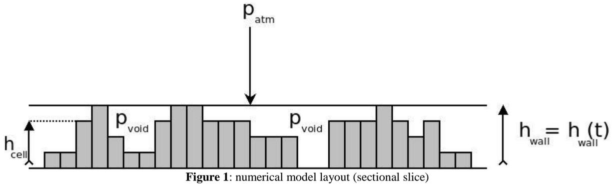
Gas pressure is found within voids through an ideal gas relationship, in a manner that allows gas voids to split or merge, whilst preserving total mass of entrapped gas. The motion of the resin is fully coupled to the gas pressure field, so voids can expand and force the fluid back from the void if the pressure is sufficiently high.
