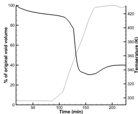
**Figure 3:** void percentage and temperature during curing. Note an initial non-physical transient for <5min has been removed.
