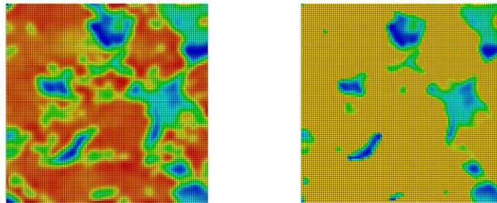
**Figure 2:** resin height distribution before (left) and after (right) compression process. Red – high fluid height, blue – low fluid height
