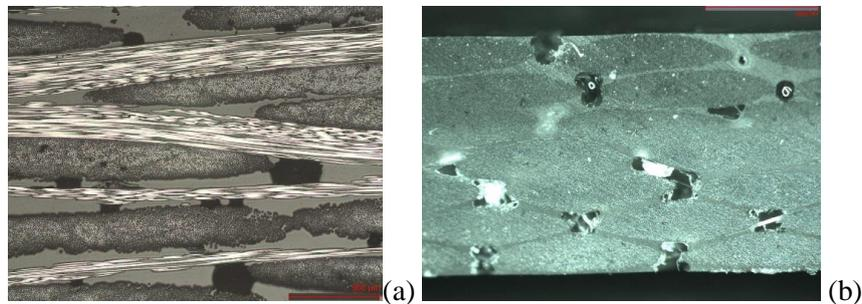
**Figure 1:** Voids presence in a carbon fibre specimen (a) and in a glass fibre specimen (b).
