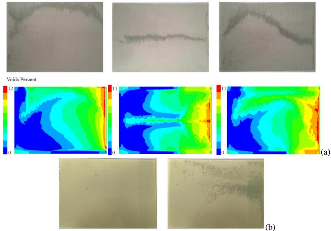
**Figure 2:** Simulation and test comparison of three glass plates infused under the same infusion conditions, varying the entity of race tracks along the edges (a). Presence of porosity in a plate with local compaction, infusion with and without vacuum condition
