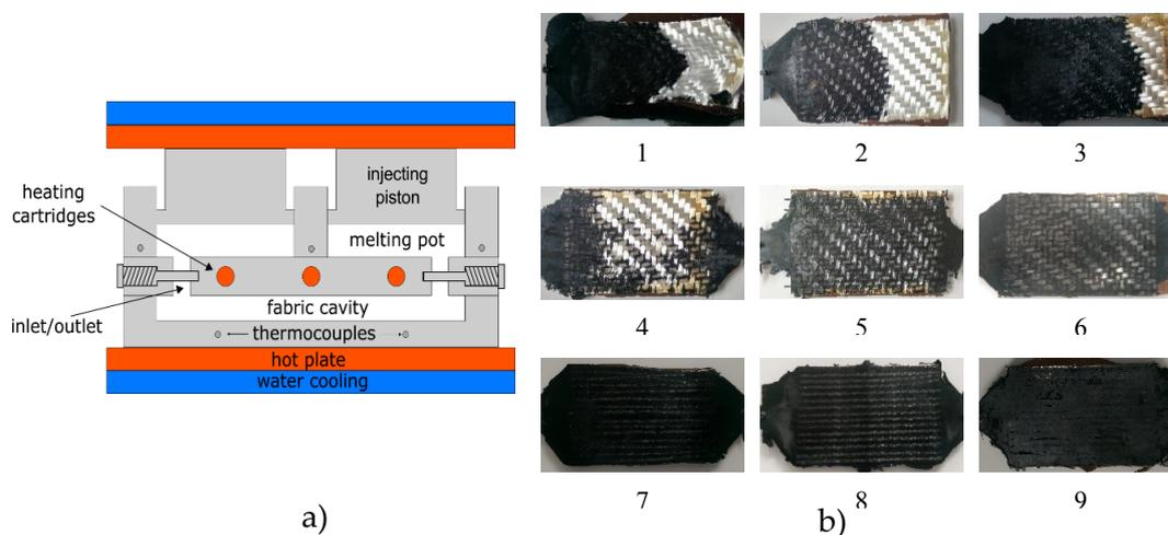
**Figure 1:** a) Schema of mold for impregnation. b) Plates produced (see Table 1 for samples' labeling).
