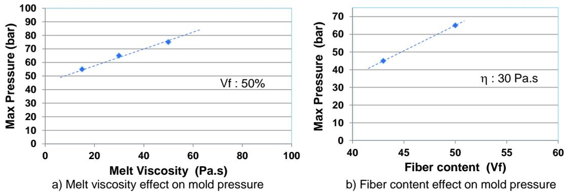
**Figure 1:** Evolution of max pressure  $P$  (compression) with melt viscosity  $\eta$  a) and fiber content  $V_f$  b) PA6 and plain glass preform system
