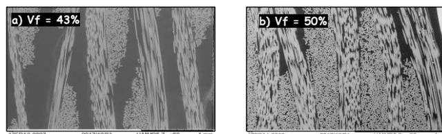
**Figure 2:** Microstructure of C-RTM TP plates obtained from low viscosity PA6 and plain glass preform (low viscosity PA6 ;  $15 < \eta < 50$  Pa.s) : a) 43% vol. fibers ; b) 50% vol. fibers).
