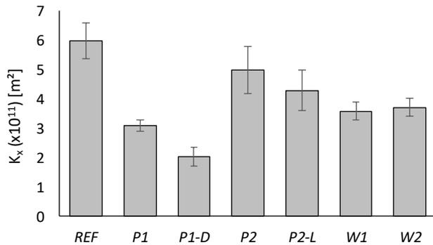
**Figure 1:** Summary of measured in-plane permeability  $K_x$ .
