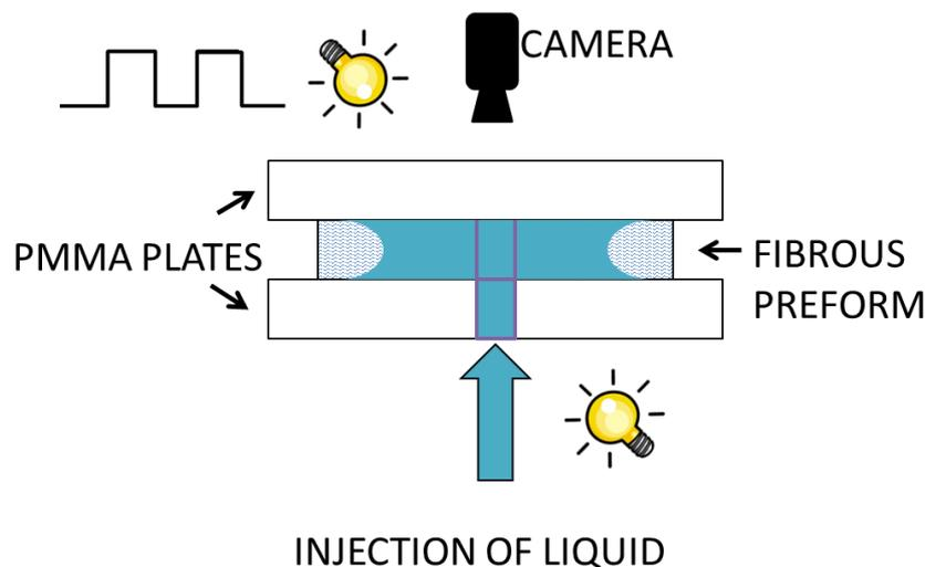
**Figure 1:** A schematic drawing of the experimental set-up designed to study the liquid front propagation in a fibrous preform during the impregnation process.
