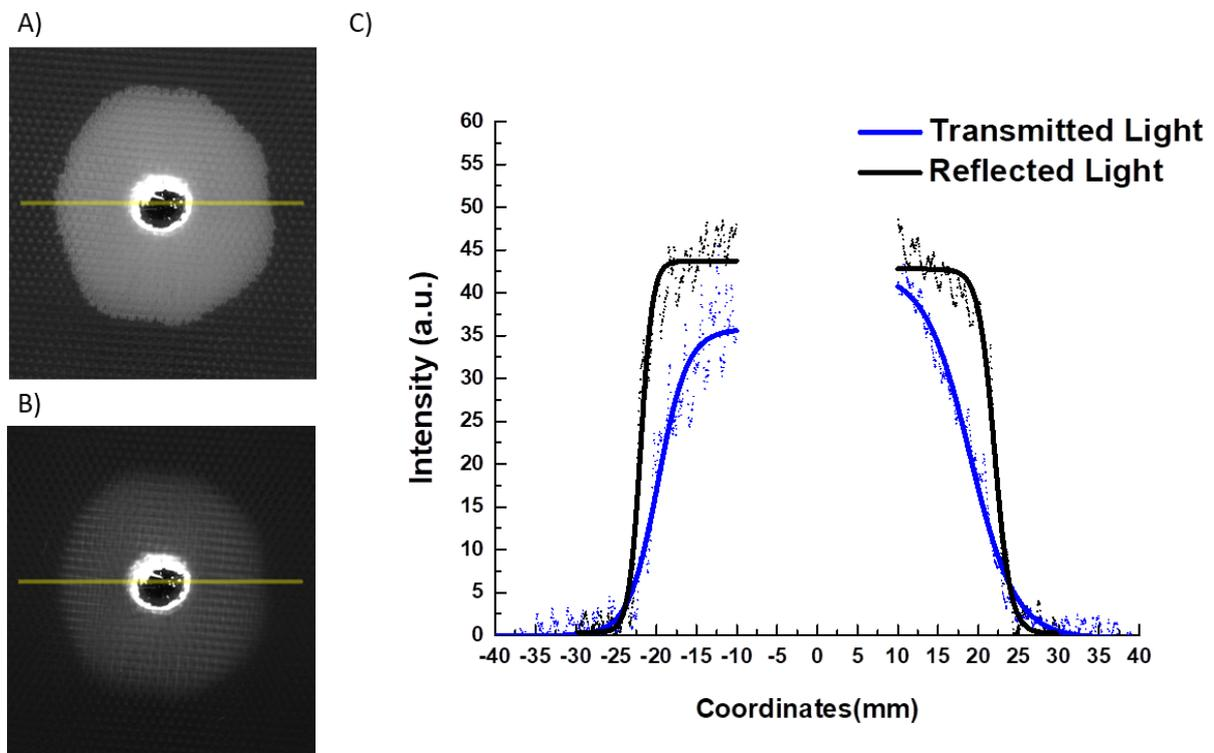
**Figure 2:** Images of the fibrous preform in reflected (A) and transmitted (B) light during the impregnation process. (C) The intensity of transmitted and reflected light along the lines shown in A and B images.
