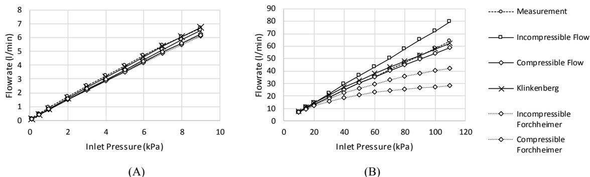
**Figure 3:** Evolution of flow rates depending on various analytical models; (A) low flow, (B) high flow.
