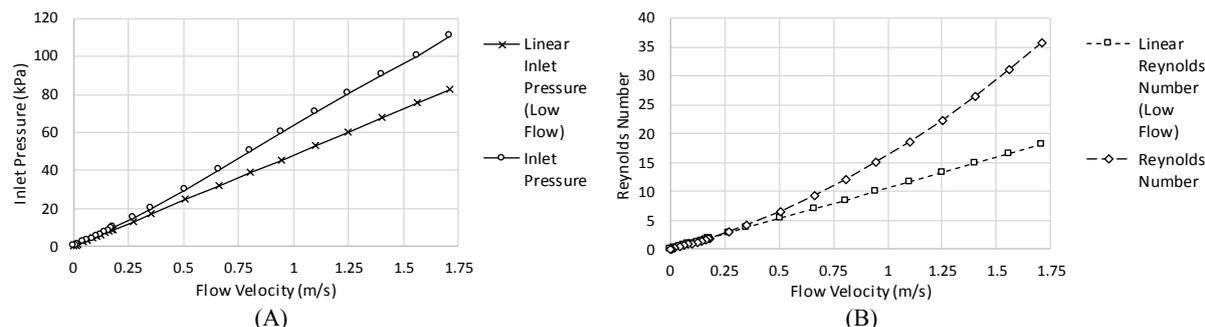
**Figure 2:** Evolution of inlet pressure (A) and Reynolds number (B) with increasing velocity.
