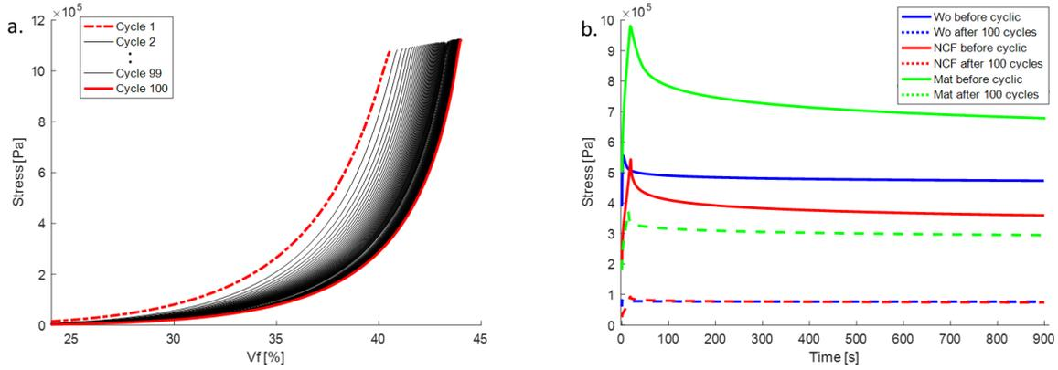
**Figure 1:** Cyclic compaction curves (Mat textile) (a). Final compaction step before and after preconditioning (b).
