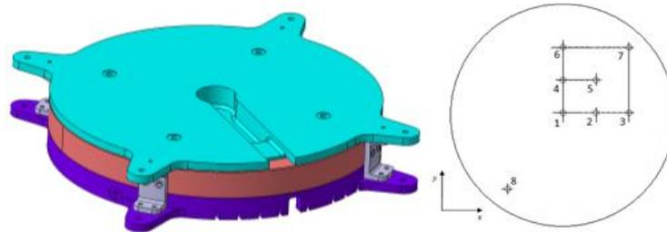
**Figure 2:** Example of instrumented RTM mould (left) and lower mould sensor setup schematic (right)
