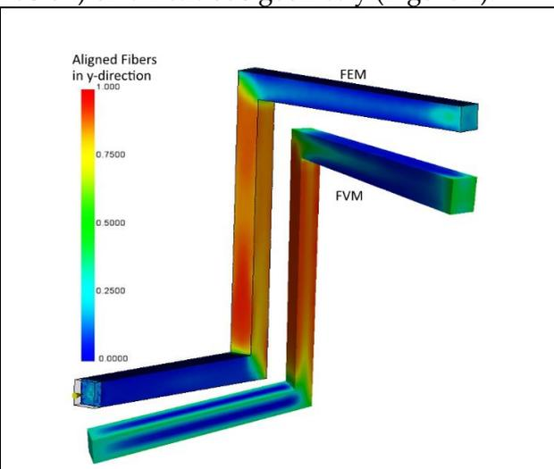
**Figure 2:** Comparison of predicted fiber orientation between FEM and FVM in y-direction [5].
