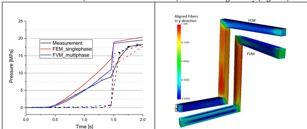
**Figure 1:** Pressure over time for a filling speed of 137.5 cm<sup>3</sup>/s and a mold temperature of 170 °C. Comparing measurement (black), FEM (red) and FVM (blue) at sensor position 1 (solid line) and 2 (dotted line) [5].
