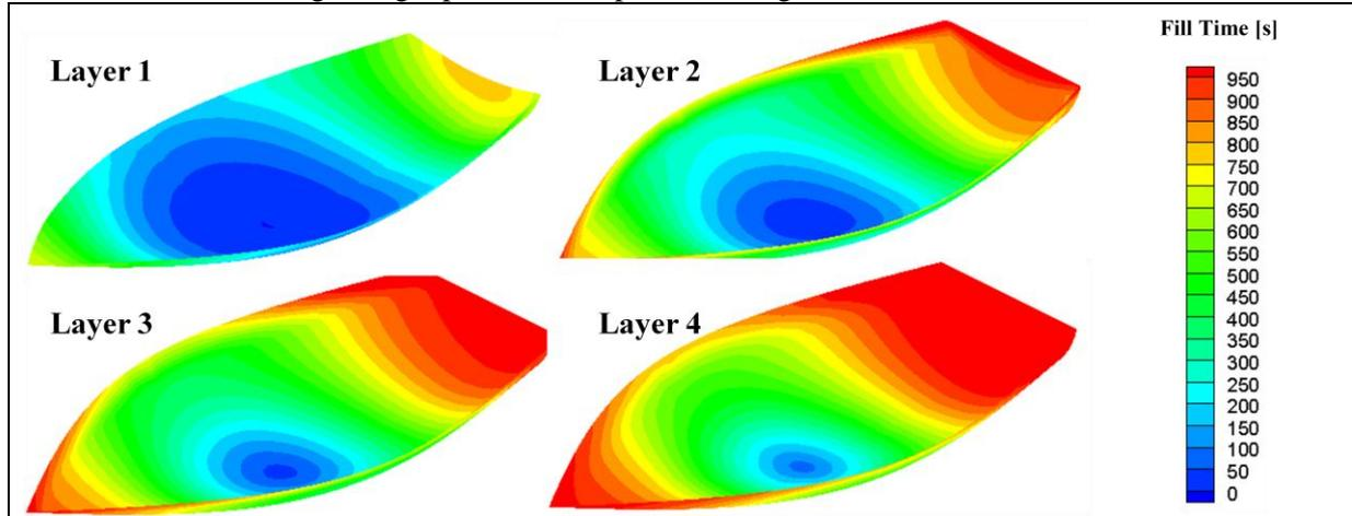
Figure 2: Mold filling pattern in the VARTM of boat structure (Layer 1: distribution medium, Layers 2-4: preform).
