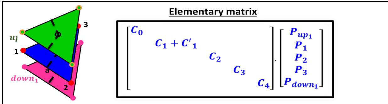
Figure 1: Elementary matrix for node 1 in the control volume finite element formulation
