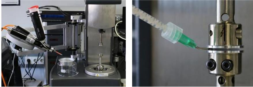
**Figure 1:** Automated specimen preparation setup: dosing and mixing unit attached to rheometer (left) and injection of the resin into the gap of the preheated parallel plate setup (right).
