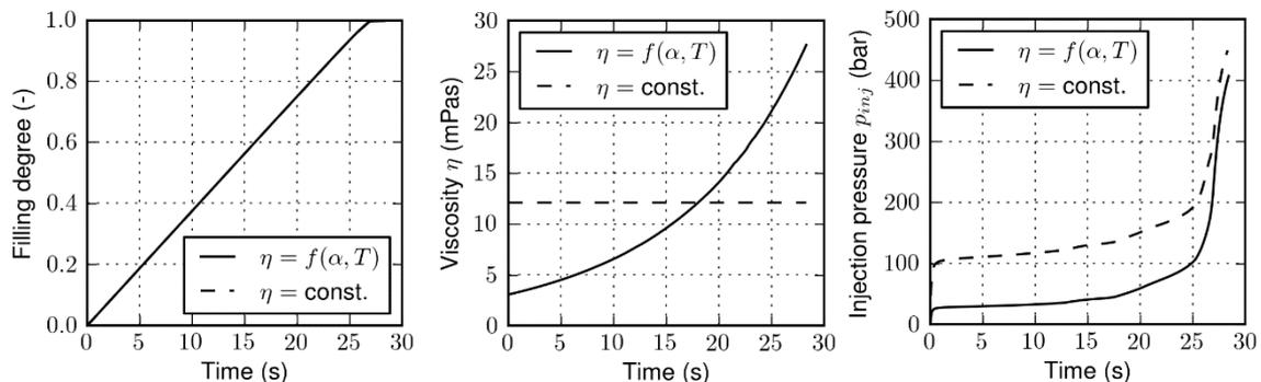
**Figure 2:** Temporal evolution of filling degree, viscosity and pressure of mold filling simulations.
