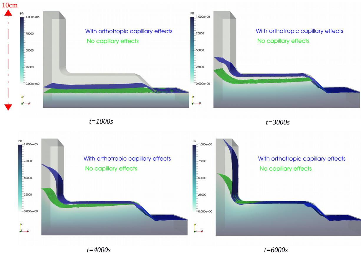
**Figure 1:** The LRI filling stage with (blue) and without (green) taking into account the capillary effects, at various time.
