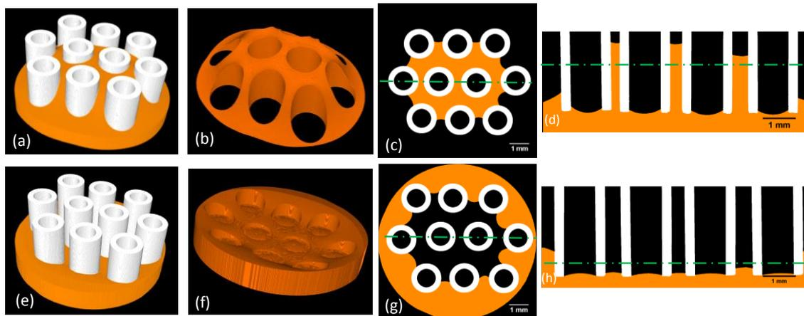
**Figure 2:** (a) 3D view of a model network made of capillary tubes (white) impregnated with distilled water (orange) obtained using X-ray microtomography imaging (voxel size of  $5.1^3 \mu\text{m}^3$ ). (b) Corresponding 3D view of the flow front between the capillary tubes. (c,d) Corresponding horizontal and vertical cross sections. First row: case of non-treated tubes. Second row (e-h): same type of views as (a-d), but for the case of Si-F treated capillary tubes.
