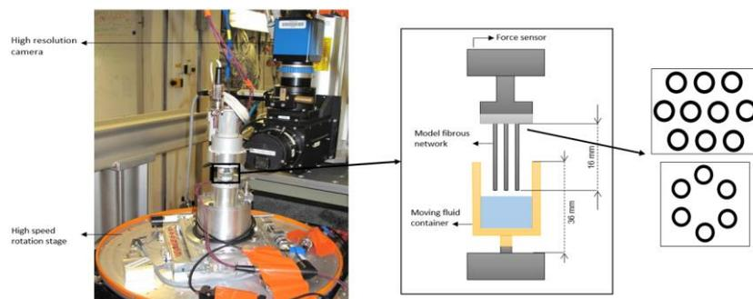
**Figure 1:** Photograph of the mini impregnation device that was installed on the microtomograph of the ID19 beamline at ESRF (Grenoble, France) and example of two different architectures of the fabricated model networks of parallel capillary tubes. Note that the tubes were sealed at their upper extremities.
