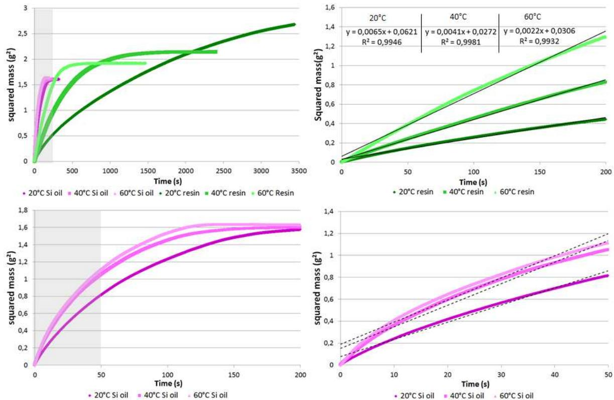
Figure 1: Wicking in quasi-UD carbon fabric along the fibres main direction with silicon oil and epoxy resin.
