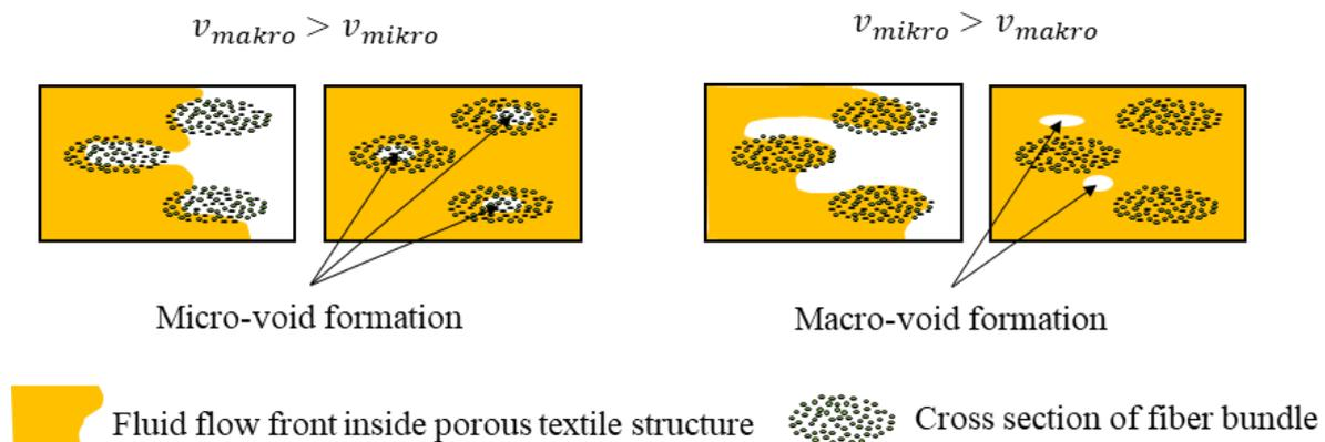
**Figure 1:** Void formation mechanisms in dual-scale porous textile: advanced macroscopic flow through inter-tow pores (left), advanced microscopic flow through inter-tow pores (right).
