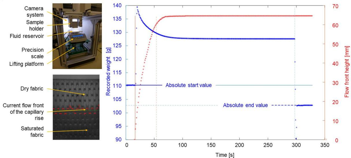
Figure 2: Set-up for vertical wicking tests (left) and capillary rise detection by image processing (right).
