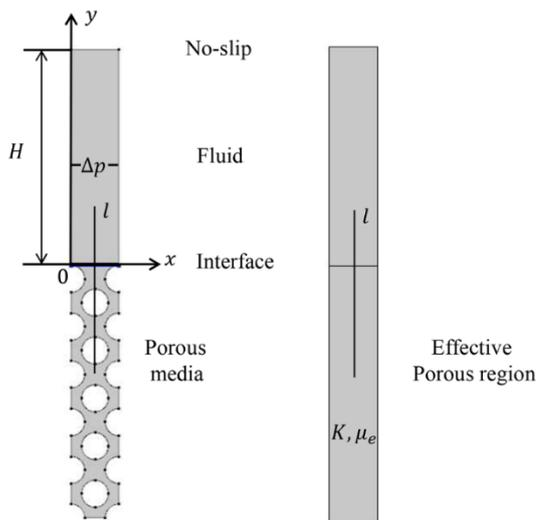
Figure 1: A schematic description of 1D transverse flow
