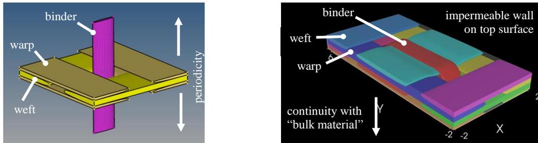
**Figure 1:** Examples of representative volume elements of “bulk material” (left) and “surface material” (right).
