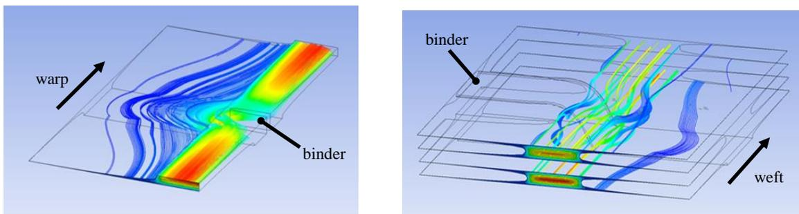
**Figure 2:** Examples of “bulk flow” (left) and “surface flow” (right), simulated for the geometries in Figure 1; colour of stream lines indicates local flow velocity.
