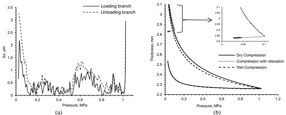
Figure 1: Typical dry and wet compaction measurements: (a) Difference between the actual compaction curve without a sample and its polynomial regression used in the data processing; the extremities were excluded in the data processing; (b) Compression curves obtained in dry compression, wet compression and wet compression with relaxation stage at 1 bar: a) relaxation test in detail, the thickness decrease during relaxation stage is progressive and reaches its maximum at the end of the stage.
