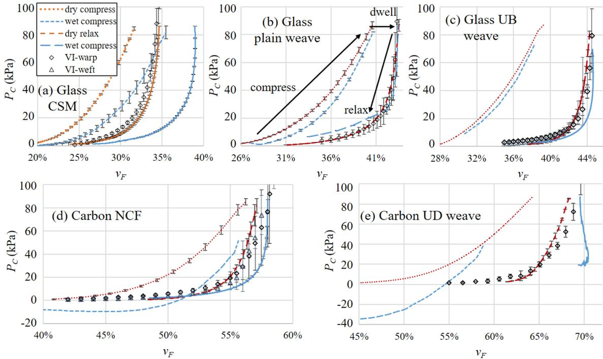
**Figure 1:** Compressibility as determined by UTM (both compaction and relaxation) and VI (wet relaxation).
