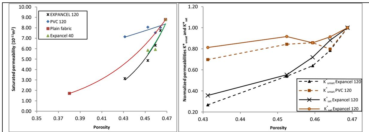
**Figure 1:** (a) Saturated permeability values (b) A comparison between the permeability values for the rigid and hollow microsphere, normalized to the plain fabric ones ( $k^*_{unsat}$  and  $K^*_{sat}$ )
