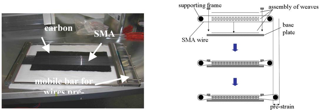
Fig. 1 Metallic frame for SMA wires positioning and procedure for pre-strain
