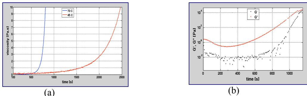
Fig. 2 (a) Effect of temperature on the viscosity evolution of the resin, (b) Evolution of elastic and viscous shear moduli of the resin at 70°C.
