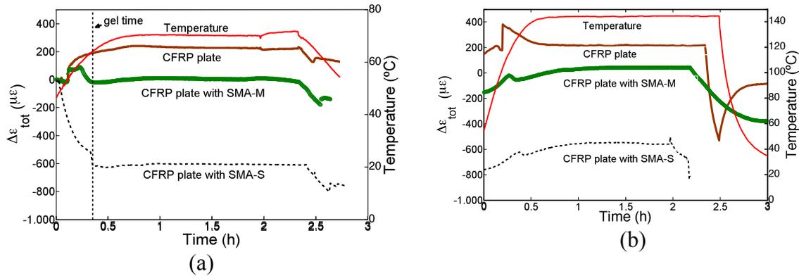
Fig. 4 Strain evolution along (a) cure and (b) post-cure
