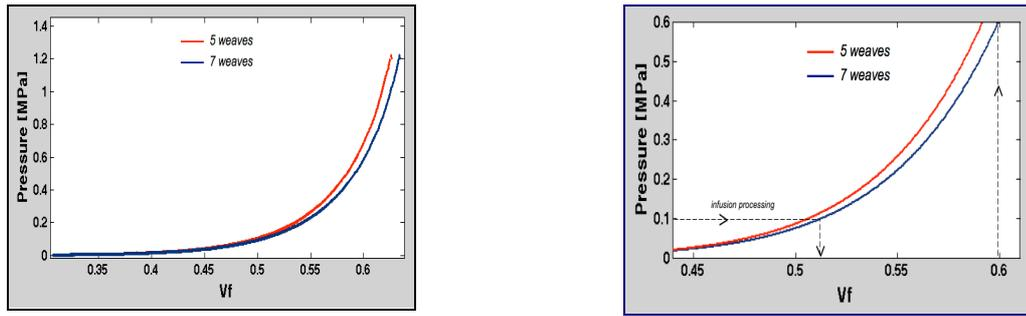
Fig.3 Results of dry compression on 5 HS weaves, with a stack of 5 or 7 weaves (0/90 and +45/-45 plies alternated)
