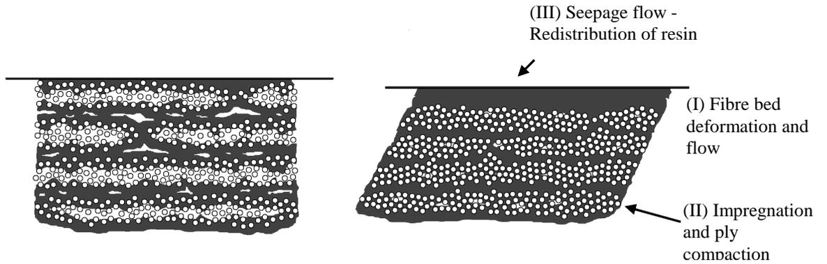
Fig. 1 The assumed manufacturing operation
