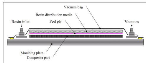
Fig. 1: Implementation of composite part manufactured by LRI process
