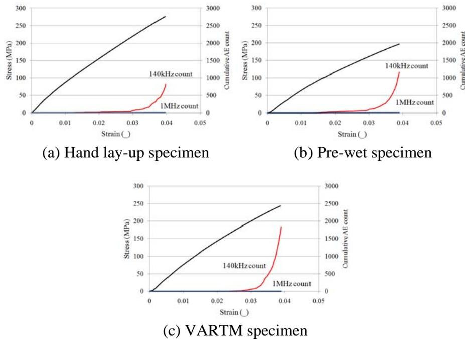
Fig. 2 Stress-strain curves
