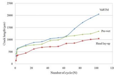
Fig. 5 Crack length of each cycle in each specimen
