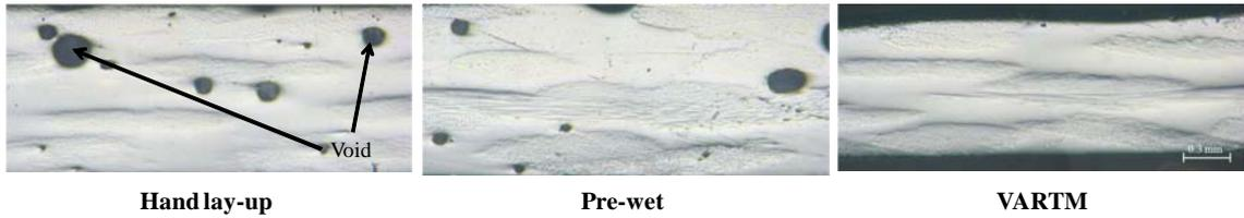
Fig. 1 Cross section of composite with different molding method
