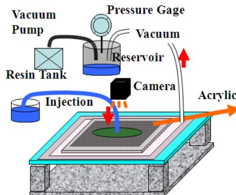
Fig.3 Experimental equipment.
