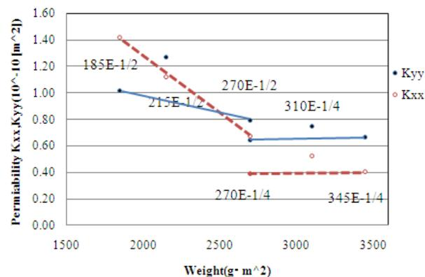
Fig.5 Relationship between permeability and weight.
