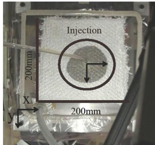
Fig.4 Resin impregnation during testing
