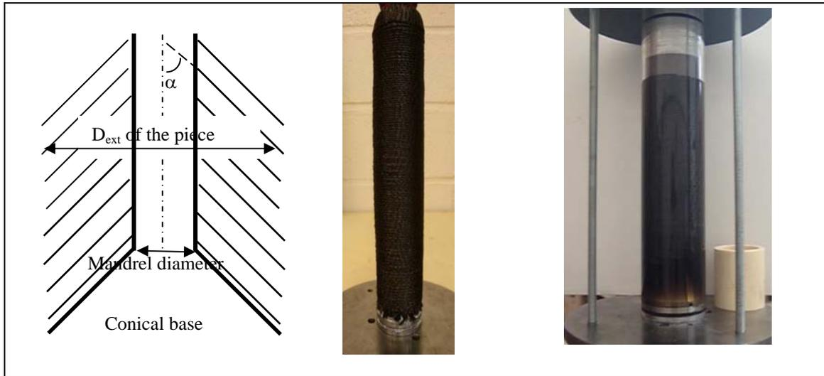
Fig. 1 (a) Scheme of the preform; (b) Final preform; (c) Resin evolution
