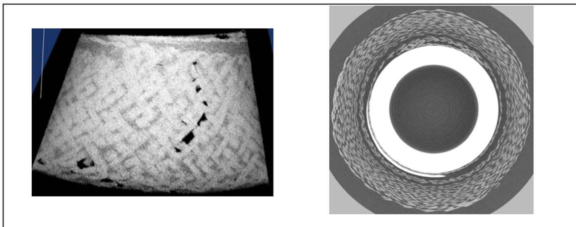
Fig. 2 (a) Position of yarns on a ply; (b) tomography to estimate the density
