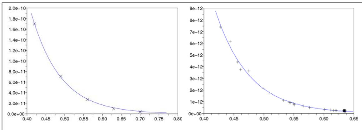
Fig. 3 (a) Planar and (b) transverse Permeability ( $m^2$ ) as a function of the fibre volume fraction
