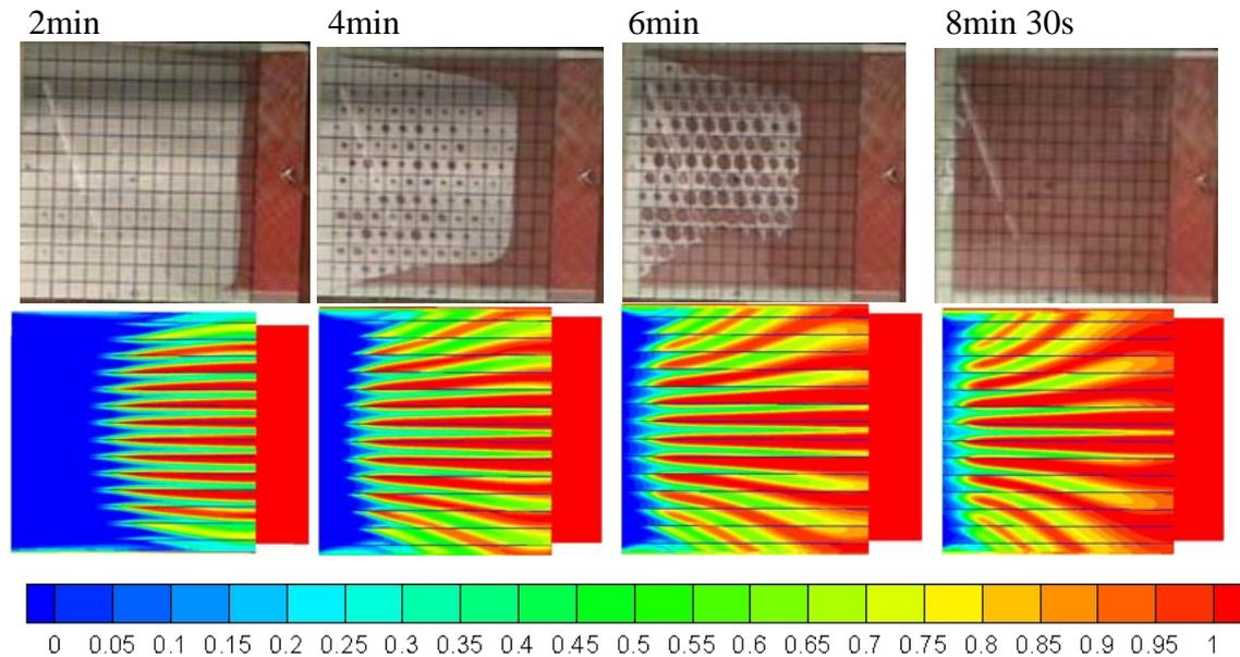
Fig.4. Flow patterns on the bottom surface of the hybrid preform.
