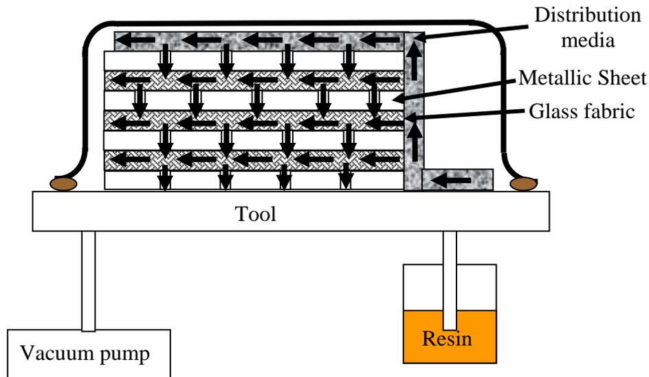
Fig. 1 Diagram of the FML VARTM process
