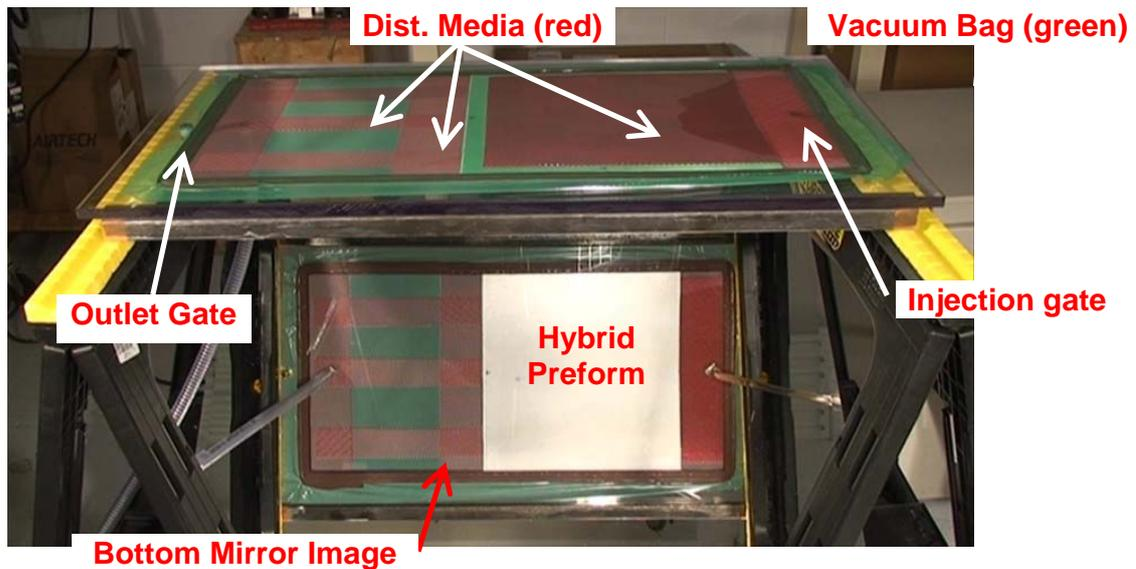
Fig. 2 Flow visualization fixture
