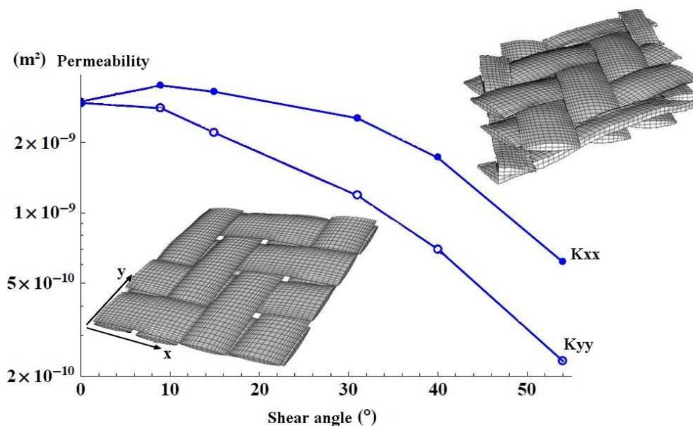
Fig. 1 Undeformed and deformed 2x2 carbon twill and influence of shear angle on permeabilities on x and y directions [10]
