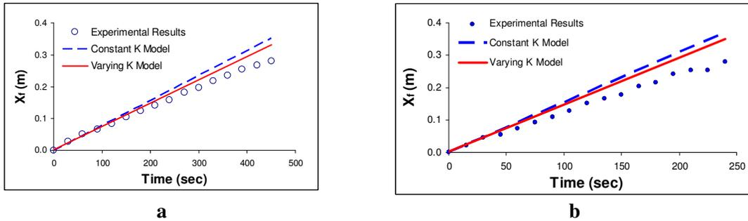
Figure 3. Flow-front position versus time plot for the flow rates of a)  $Q = 1 \text{ mL/s}$  and b)  $Q = 2 \text{ mL/s}$
