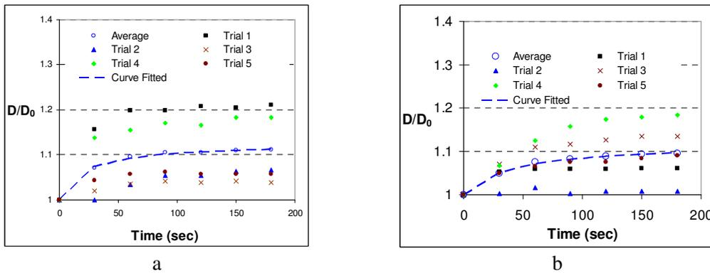
Figure 2. Swelling diameter as function of time for a) broken wood fibers and b) unbroken wood fibers. (The fibers are wetted by the water-diluted corn syrup.)
