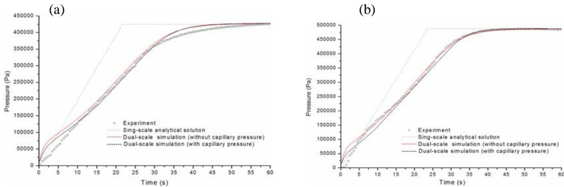
Figure 2: Comparison of the experimental inlet-pressure history with the numerical predictions: (a) the x-direction flow; (b) the y-direction flow.
