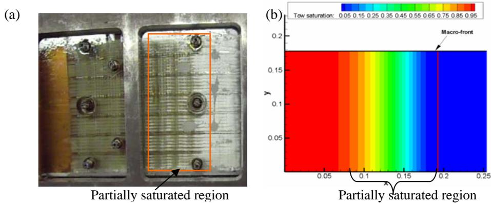
Figure 3: Snap shots of the tow-saturation distributions at  $t = 24s$  during the 1-D flow experiment: (a) from the experiment; (b) from the dual-scale mold-filling simulation.
