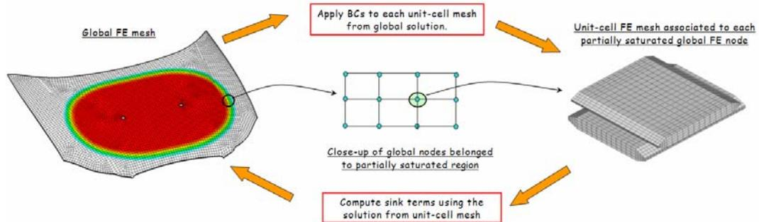
Figure 4: Relation between the global and local unit-cell FE models.
