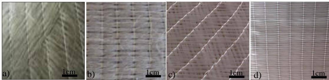
Fig. 1 Biaxial (a) and unidirectional (b) flax fabrics; biaxial (c) and unidirectional (d) glass fabrics
