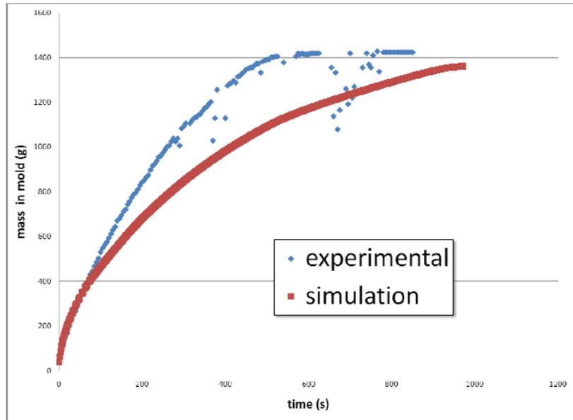
Figure 7: Comparison of experimental and simulated resin injection into the mold
