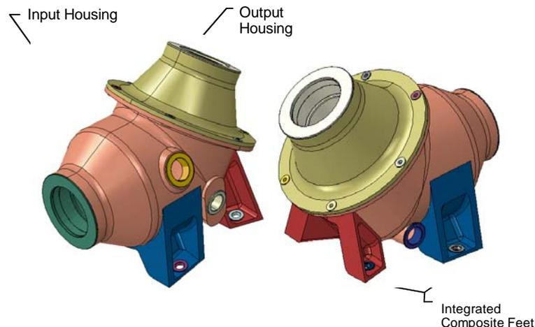
Figure 1: Final Gearbox Housing Design
