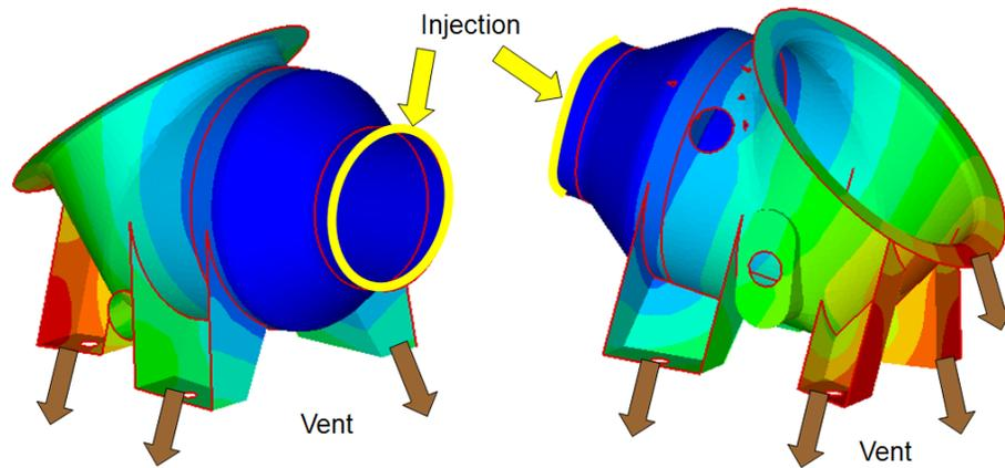
**Figure 4: The results of the flow simulation for the input housing. Different colors indicate different times of resin arrival.**
