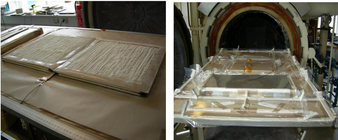
Fig. 1 Lay-up and the oven (in this case an autoclave) used for the vacuum consolidation process
