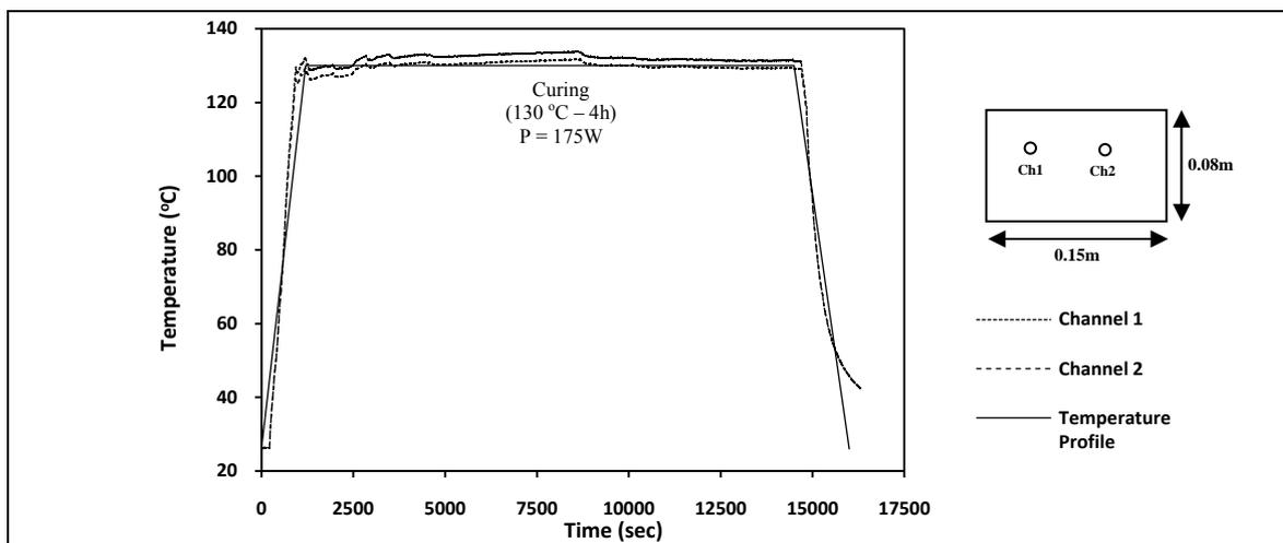
Fig. 3 Temperature distribution in UD Sigrafil/E022 prepreg
