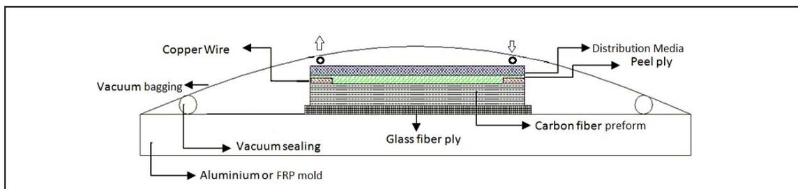
Fig. 1 Setup using the SCRIMP method and Resistive Heating
