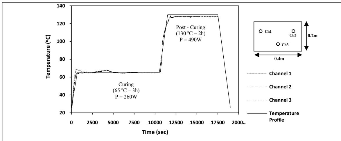
Fig. 2 Temperature distribution on CF Fabric/Epocast52 using vacuum bagging method
