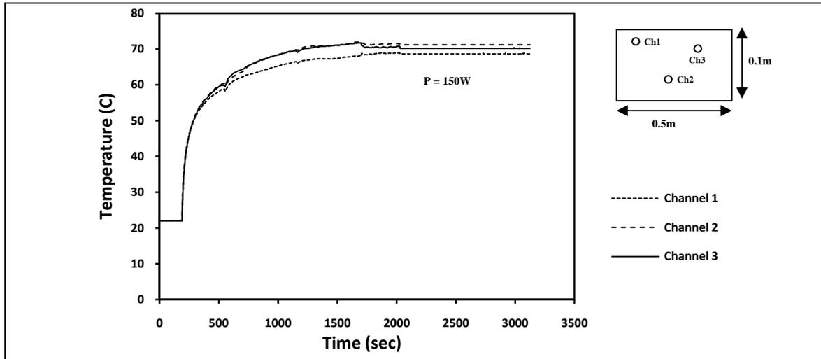
Fig. 4 Temperature distribution in UD T700S before the resin flow, using SCRIMP method
