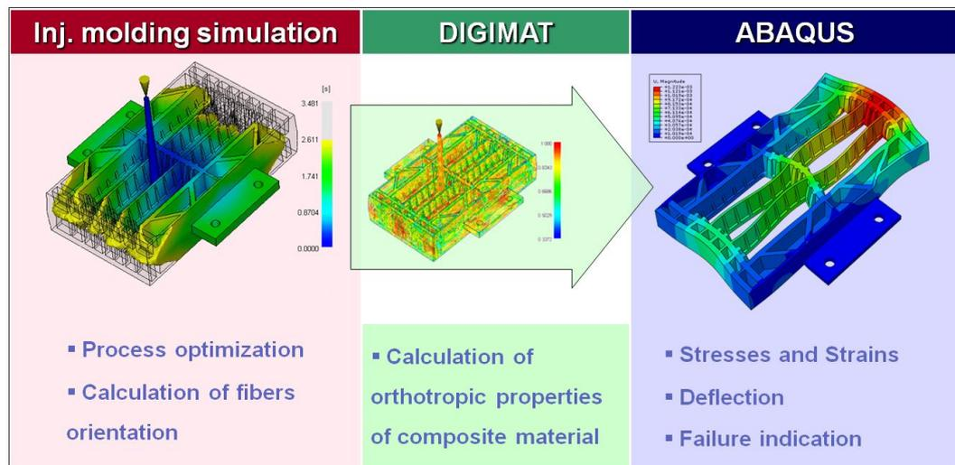
Fig. 2 Simulation approach for short fiber reinforced thermoplastics processed by injection molding
