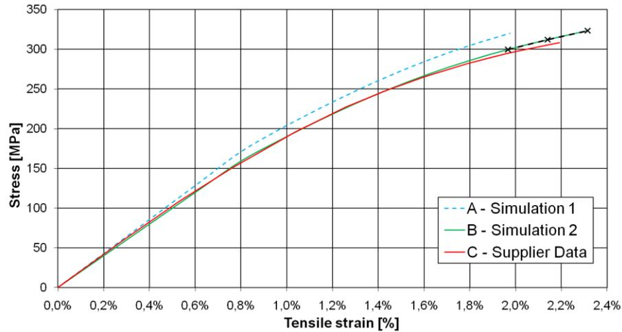
Fig. 3 Comparison of real and virtual tensile test results for directly molded ISO 527 sample made of polyarylamide reinforced with 50% glass fibers
