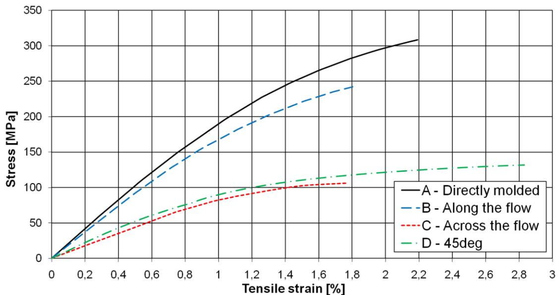
Fig. 1 Comparison of tensile test results for polyarylamide 50% glass fibers in case of different orientation of short fibers
