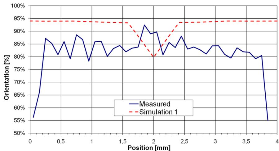
Fig. 4 Fibers orientation through thickness in directly molded ISO 527 sample (measured in the middle of the sample width)
