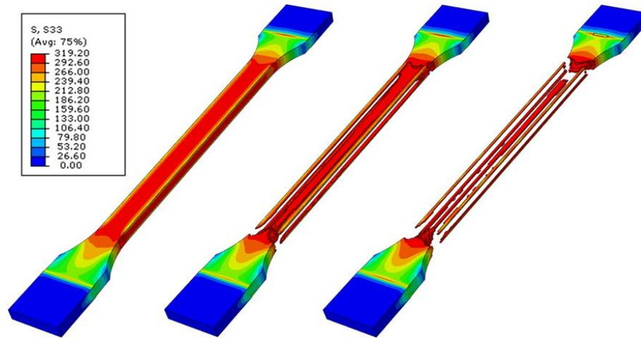
Fig. 5 Stress in ISO 527 sample at different load steps
