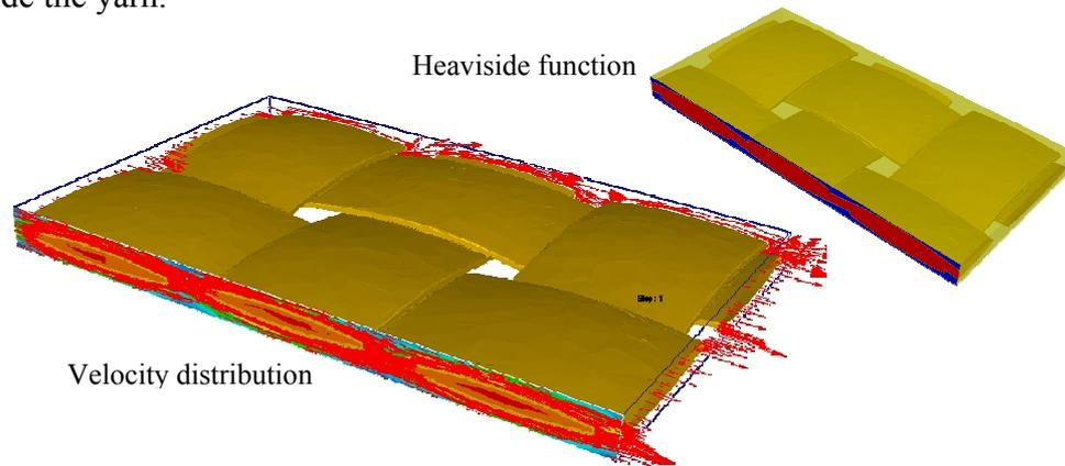
Fig. 3 Distribution of the velocity field on the half geometry defined through the immersion of one ply.
