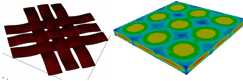
Fig. 1 Example of a computational domain at the meso scale. In the left; the yarn's meshes (courtesy of Lamcos-Insa de Lyon); on the right, the distribution of the distance function.
