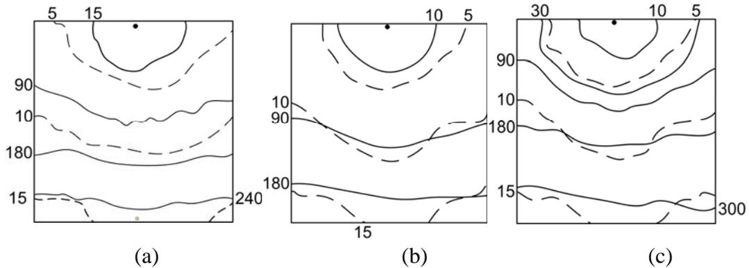
Fig. 4: Effect of varying the injection pressure. (a) normal, (b) halved (c) doubled
