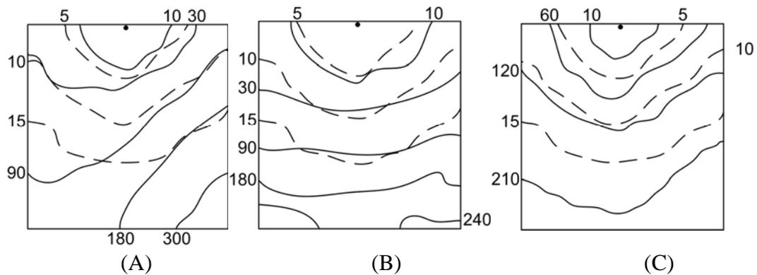
Fig. 6: Effect of varying the permeability (A) falling left to right, (B) falling top to bottom (c) rising top to bottom.
