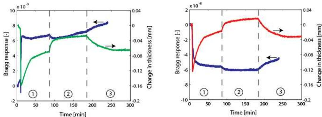
Figure 3. Bragg responses and changes in thickness for FBG 1 (LHS) and FBG 2 (RHS)
