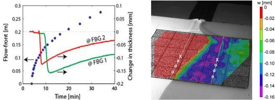
Figure 2. LHS: average position of flow-front and change in thickness close to FBGs, RHS: surface plot of change in thickness at  $t = 9.33$  min
