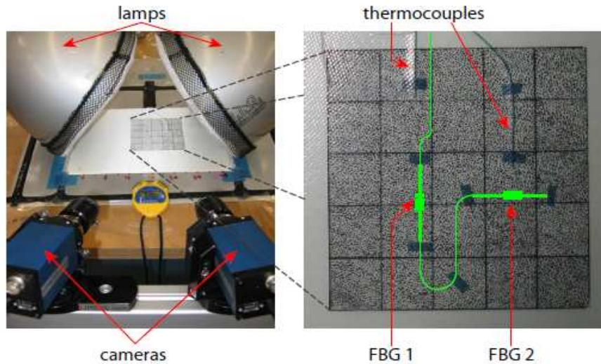
Figure 1. LHS: Experimental set-up, RHS: grid with stochastic pattern and position of sensors (path of fibre optic is highlighted in green) (right-hand side)
