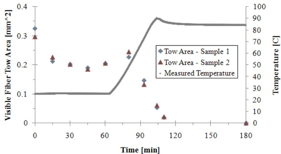
Fig. 2 Visible fibre tow area and cure cycle temperature with processing time.
