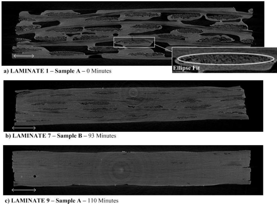
Fig. 1 X-ray micrographs of microstructural evolution (adjusted for visibility).
