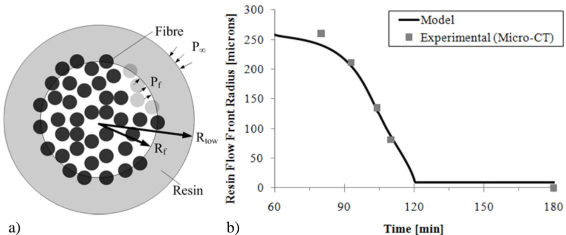
Fig. 3 a) Schematic of fibre tow approximation; b) graph of resin flow front radius versus time from experiments and modeling.
