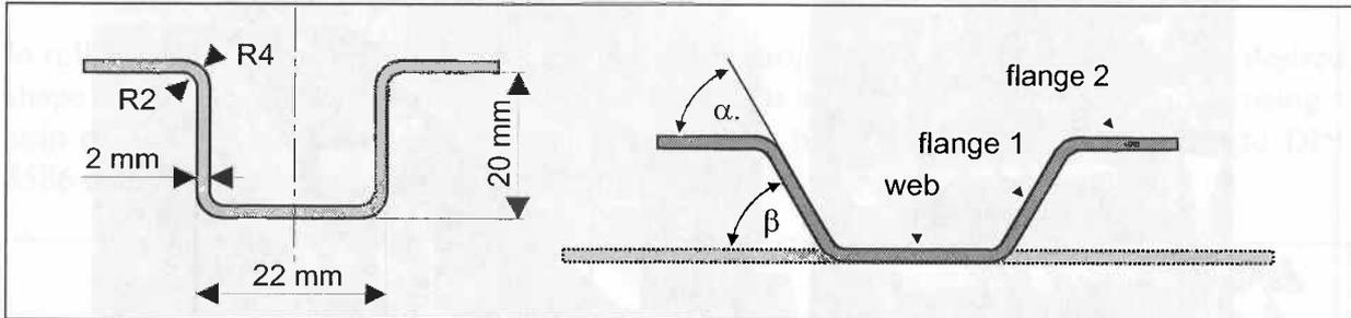
Figure 4 Dimensions and nomenclature of roll formed section
