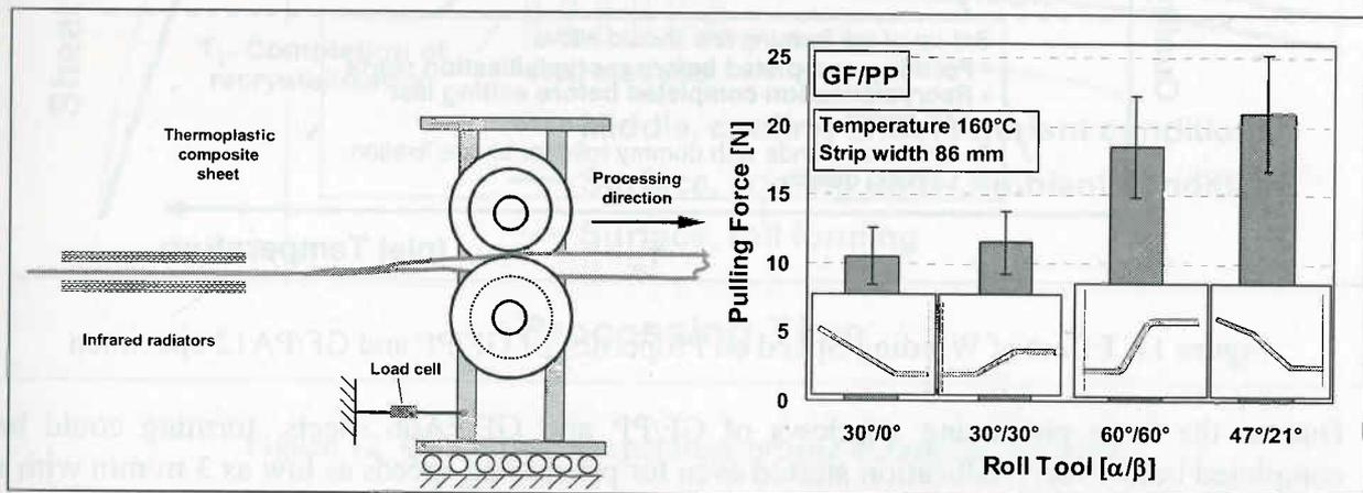
Figure 10 Schematic of the experimental set-up and influence of shaping rolls
