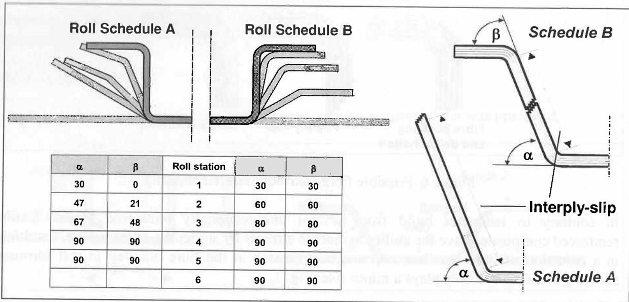
Figure 8 Flower patterns and distance over which interply-slip is required
