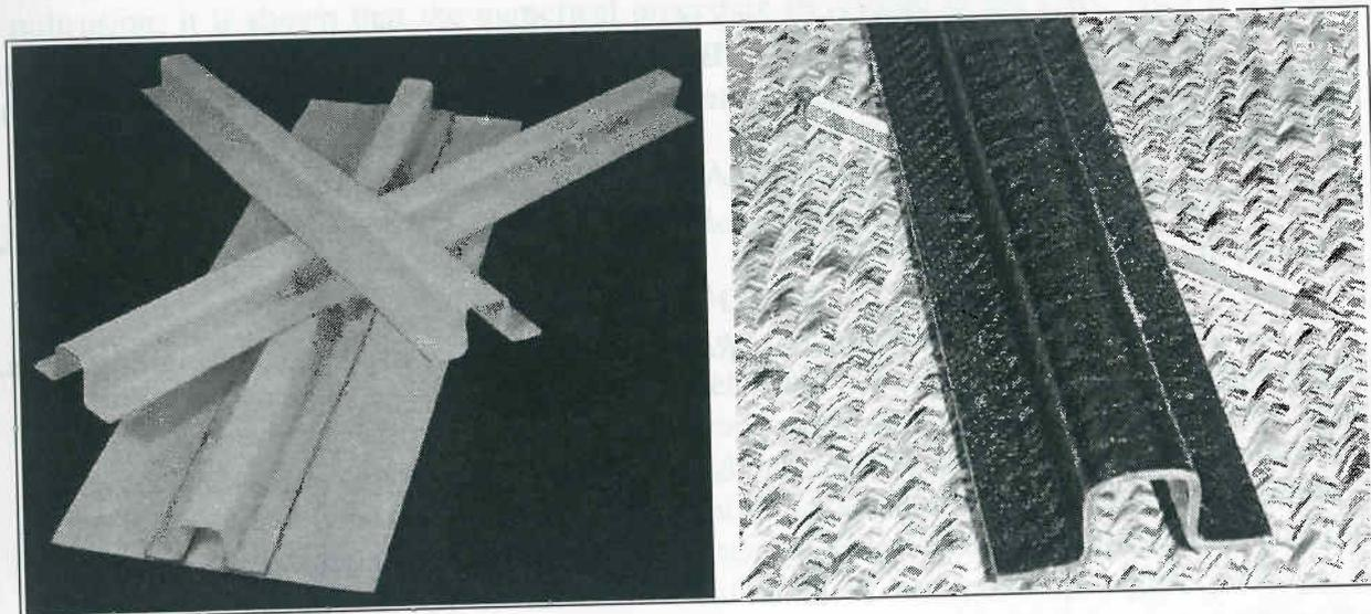
Figure 13 Roll formed GF/PP (left) and GF/PA66 profiles (right)
