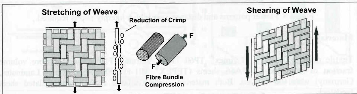
Figure 7 Deformation processes in textile reinforced composites
