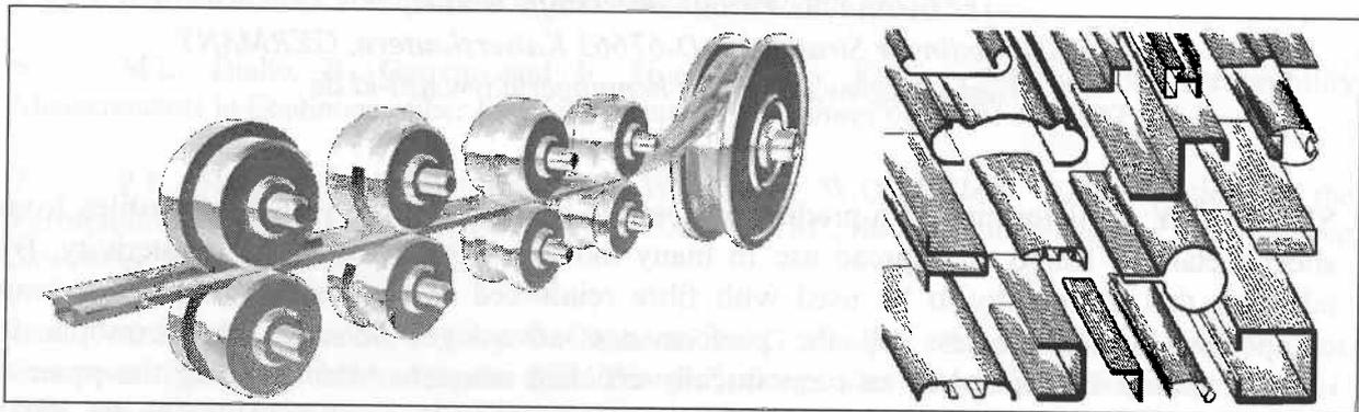
Figure 1 Schematic of roll forming operation and typical roll formed profiles
