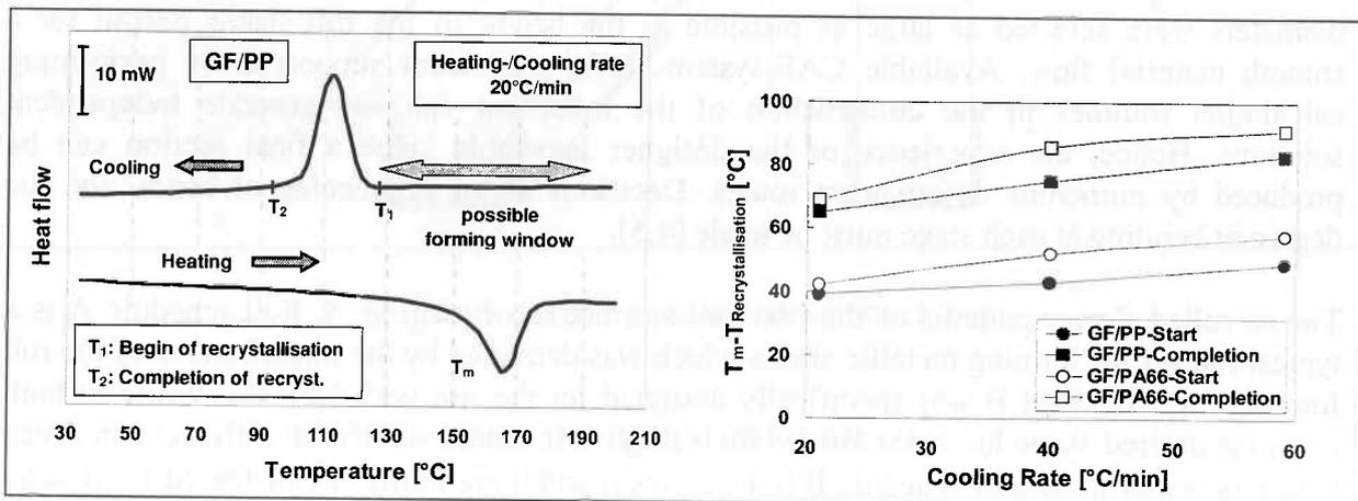
Figure 9 DSC curve of GF/PP and cooling of GF/PP and GF/PA66
