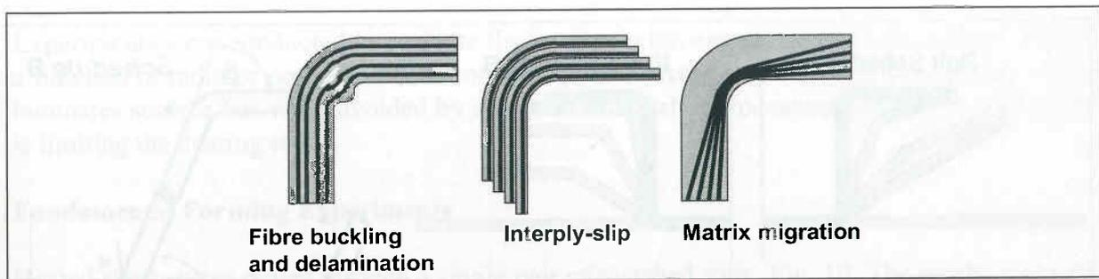
Figure 6 Possible fibre distributions after forming
