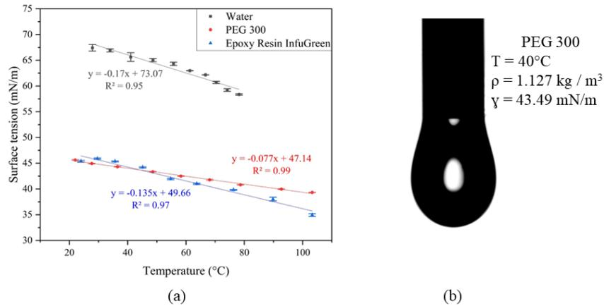
**Figure 1: (a) Surface tension against temperature, by Wilhelmy plate method; (b) Surface tension result of PEG 300 at 40°C, by Pendant Drop method.**
