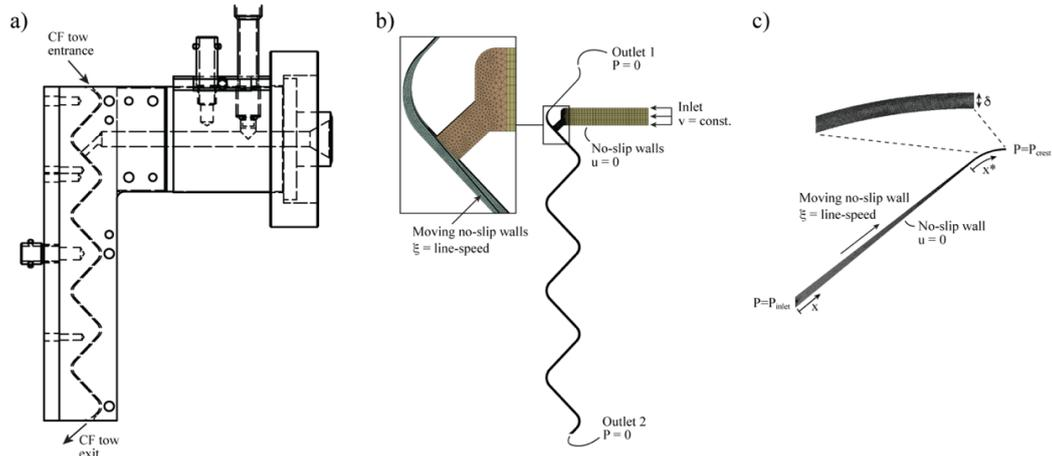
**Figure 1: (a) mechanical drawing of the cross-head melt impregnator. (b) illustration of the global impregnator domain with a carbon fibre tow entering from the top and exiting through the bottom. (c) illustration of the ‘wedge’ domain. This represents the polymer which is between the moving carbon fibre tow and the crest, where the domain contracts to the melt film thickness ( $\delta$ ).**
