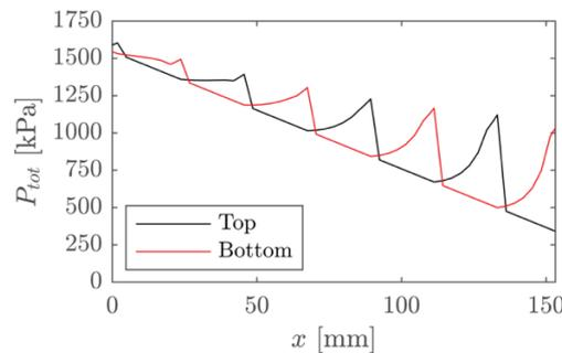
**Figure 2: Combined static, ‘wedge’ and ‘crest’ pressure for a die with seven crests, a crest spacing of 20 mm, contact angle of 41°,  $\mu = 200$  Pa.s,  $v_f = 0.6$ , and a line-speed of 0.2 m.min<sup>-1</sup>. The pressure at each crest alternates between the top and bottom of the fibre tow. Crest pressure incrementally increases due to elevated tension by contact friction.**
