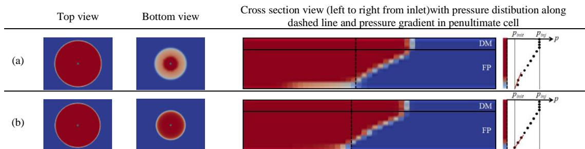
**Figure 1: Filling state after 30 s using interFoam with (a) slip wall and (b) dynamic boundary conditions.**
