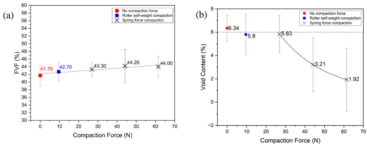
Figure 1: Impact of the on-line compaction system on towpreg FVF (%) with a small range or 2.5% deemed negligible (a) and void content (%), demonstrating a minimum threshold for compaction effectiveness and diminishing returns in void reduction with increased compaction force (b)
