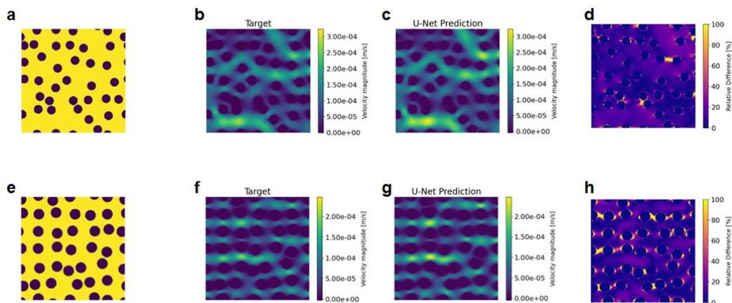
**Figure 2.** Two examples (a-d training set, e-h validation set) demonstrating the microstructures, and corresponding flow fields: b&f ground truth and c&g U-net prediction, and d&h the deviation of the U-net prediction from the ground truth.
