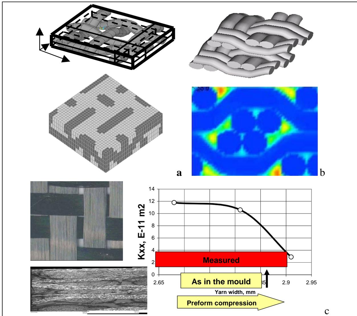
Figure 3 Calculation of permeability: (a) unit cell and voxel model; (b) Two layers of monofilament fabric: *WiseTex/LamTex* model and flow velocity field (finite difference method); (c) Carbon woven reinforcement: fabric, cross-section of the laminate ( $V_f=55\%$ ), finite element calculations with different compression of the fabric
