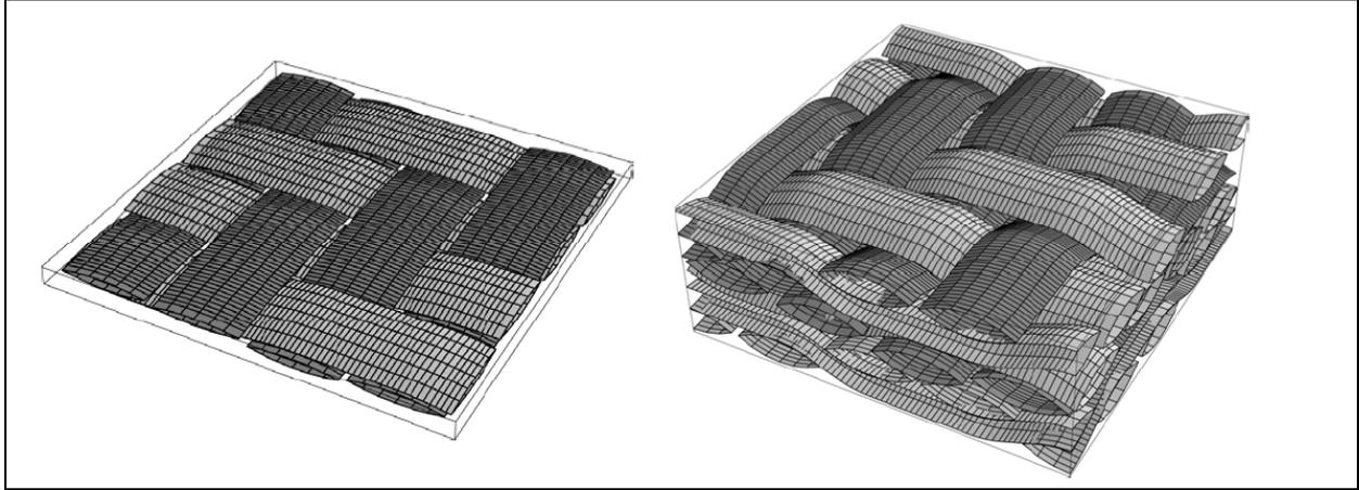
Figure 2 FE mesh for surfaces of yarns of one layer of woven fabric and a laminate
