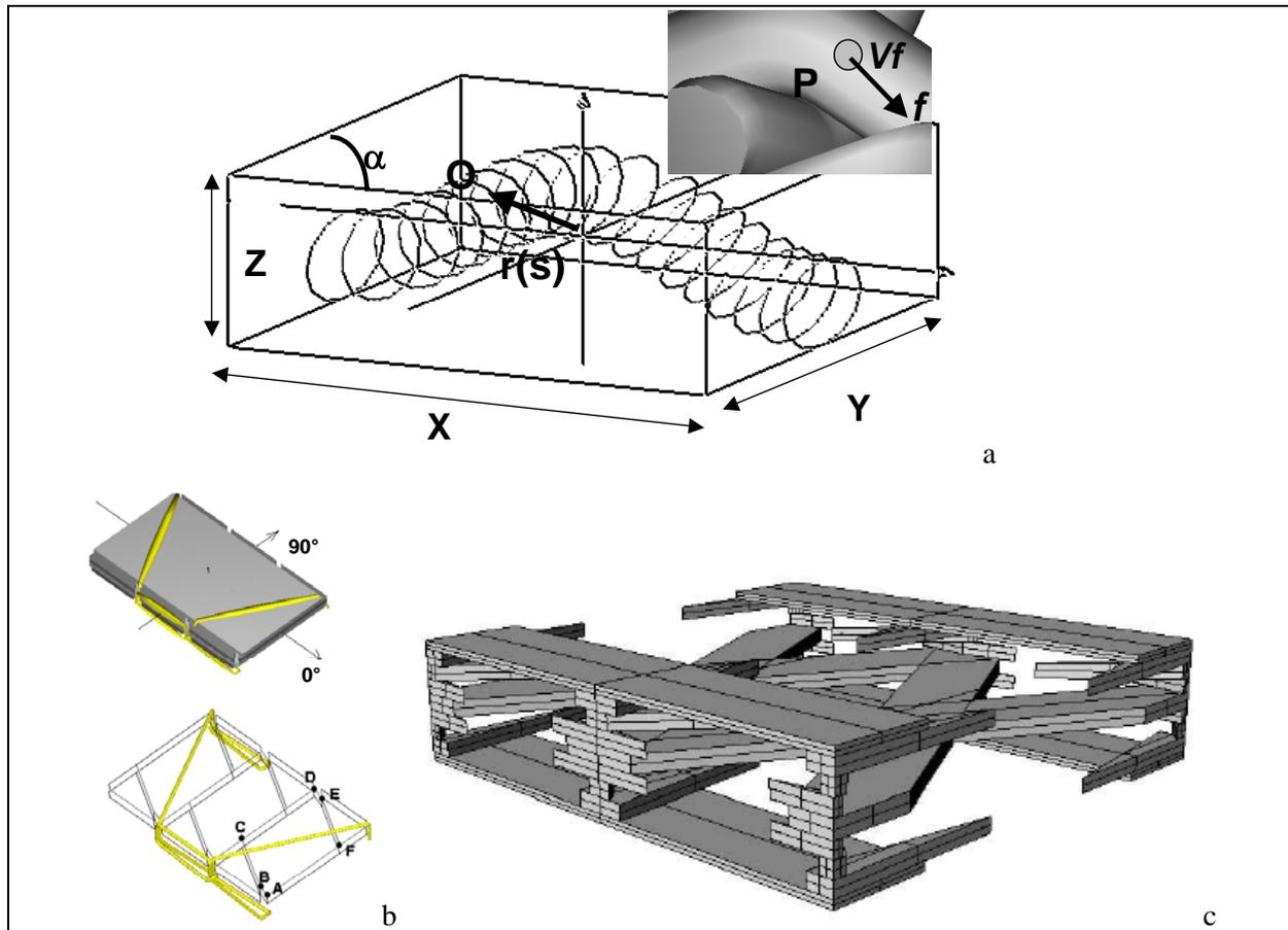
Figure 1 (a) Set of cross-sections defining a yarn in a unit cell, properties of fibres near point P; (b) Quadriaxial NCF, orientation of the fibres in the plies  $0^\circ/-45^\circ/90^\circ/45^\circ$ : Full geometrical model with stitching. Note a “channel” in the first  $0^\circ$  ply and slab representation of a ply with  $-45^\circ$  “cracks”. ABCDEF – vertices of the upper polygon of one of the slabs; (c) Example of the pore structure of biaxial NCF
