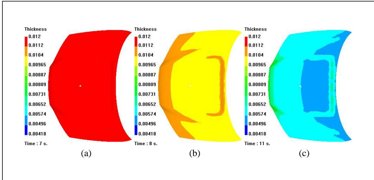
Fig. 8 Thickness variation during filling: (a) at 7 sec; (b) 8 sec; and (c) 11 sec
