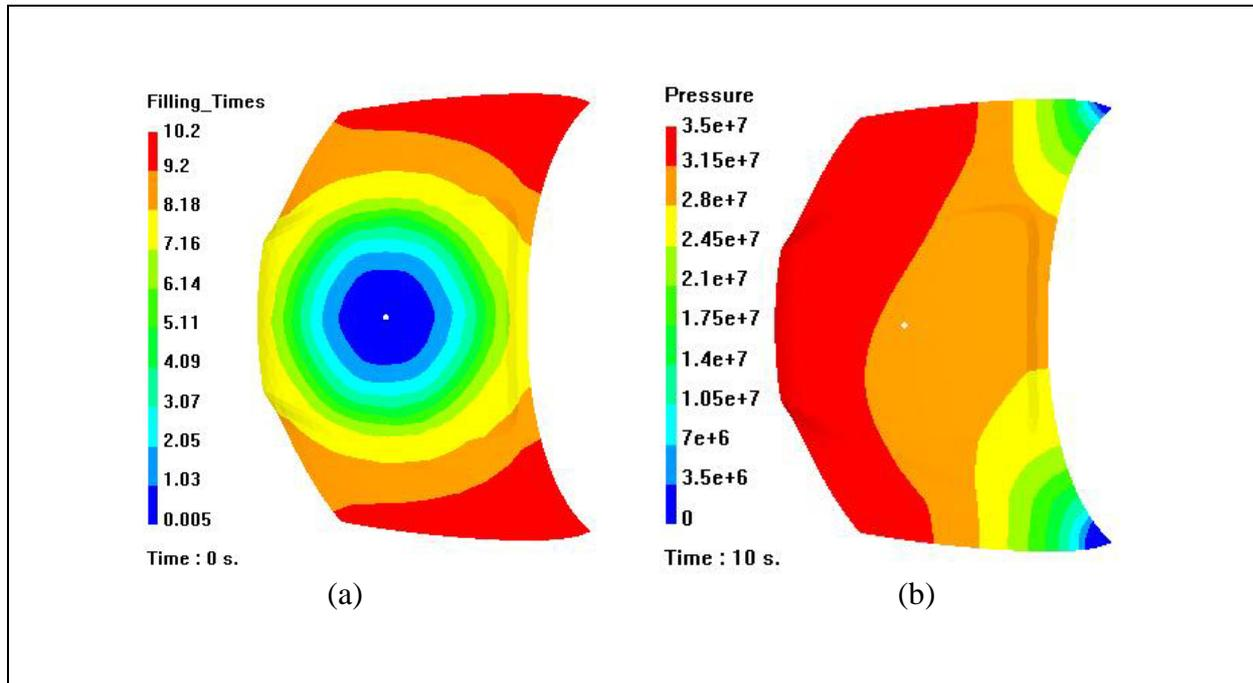
Fig. 7 Filling of the hood by the ACRTM process: (a) filling time distribution; (b) pressure distribution
