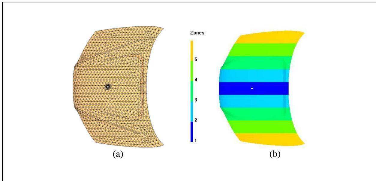
Fig. 3 The mold cover is split into segments in order to carry out ACRTM
