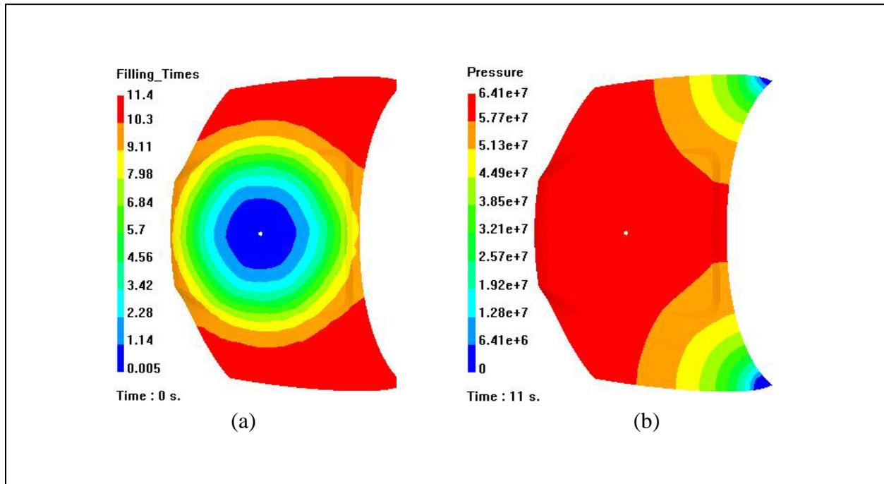
Fig. 9 Filling of the hood by the CRTM process: (a) filling time distribution; (b) pressure distribution
