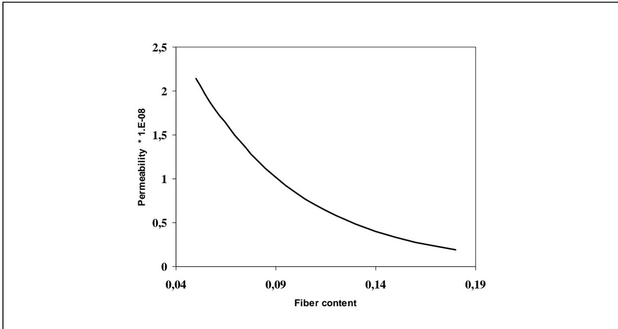
Fig. 4 Permeability vs. fiber content for the reinforcement used in the simulations
