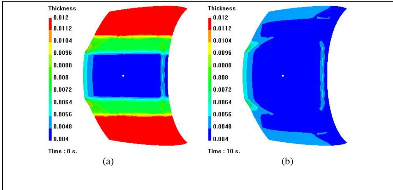
Fig. 6 Thickness variation during compression (ACRTM): (a) at 8 sec; (b) 10 sec
