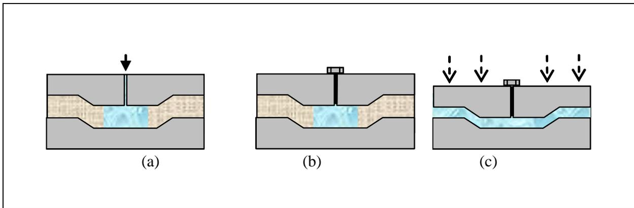
Fig. 1 Main steps of Compression Resin Transfer Molding (CRTM)
