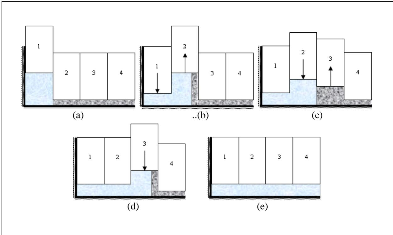
Fig. 2 Main steps of Articulated Compression Resin Transfer Molding (ACRTM)
