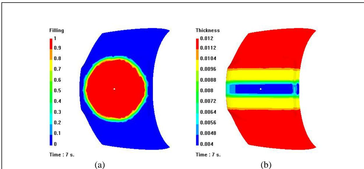
Fig. 5 Beginning of the compression process after 7 sec of filling: (a) flow front at 7 sec; (b) thickness distribution at 7 sec
